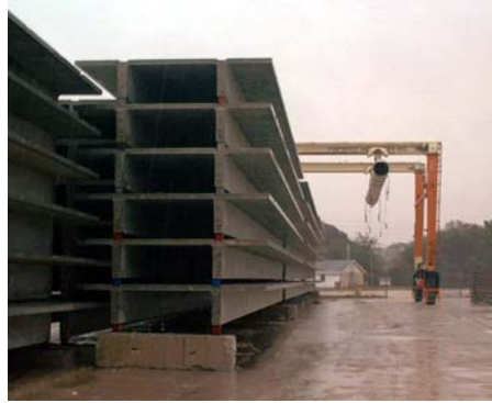
Figure 1. A stack of precast concrete double tees in a typical storage yard.
