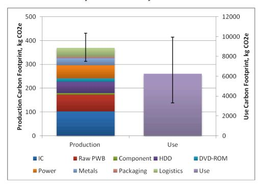
Figure 1: Product Carbon Footprint of IBM Server by Component and Phase. The production phase is presented on the left axis, use phase on the right axis.
